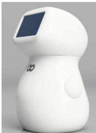
cinnamon is a self-propelled, smart robot equipped with a camera and AI functions that the user can enjoy communicating with. It can be controlled remotely via a smartphone app by pressing buttons and by voice commands. Haneda Robotics Lab will collect data with the aim of improving voice recognition efficiency in AI conversations, while providing multilingual information services for customers and remote operator connection tests.
