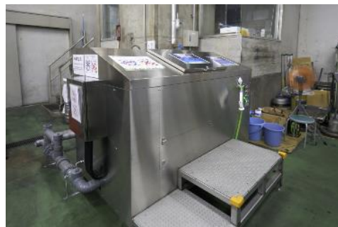
Fully automated vanishing-type food waste disposers
